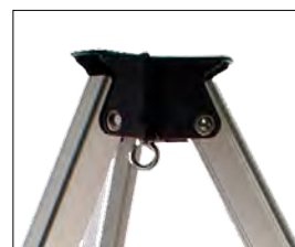
Standard IndustriPOD has a one-piece fabricated steel head with centre eyebolt and three 360kg stabilisation anchor points
